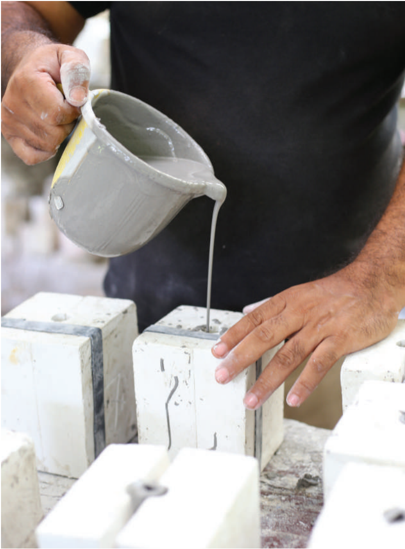
The ceramic slurry is poured into a mould in the shape of the component to be cast and left to solidify.
