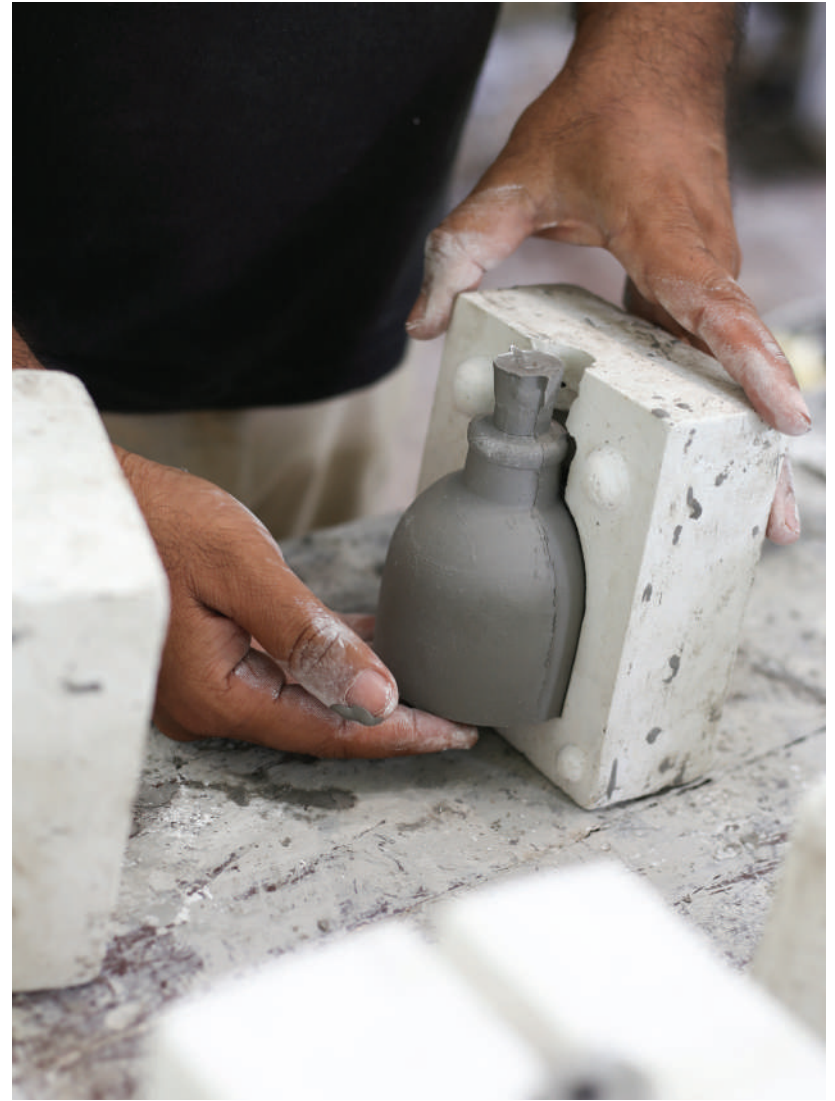
The ceramic slurry is poured into a mould in the shape of the component to be cast and left to solidify.
