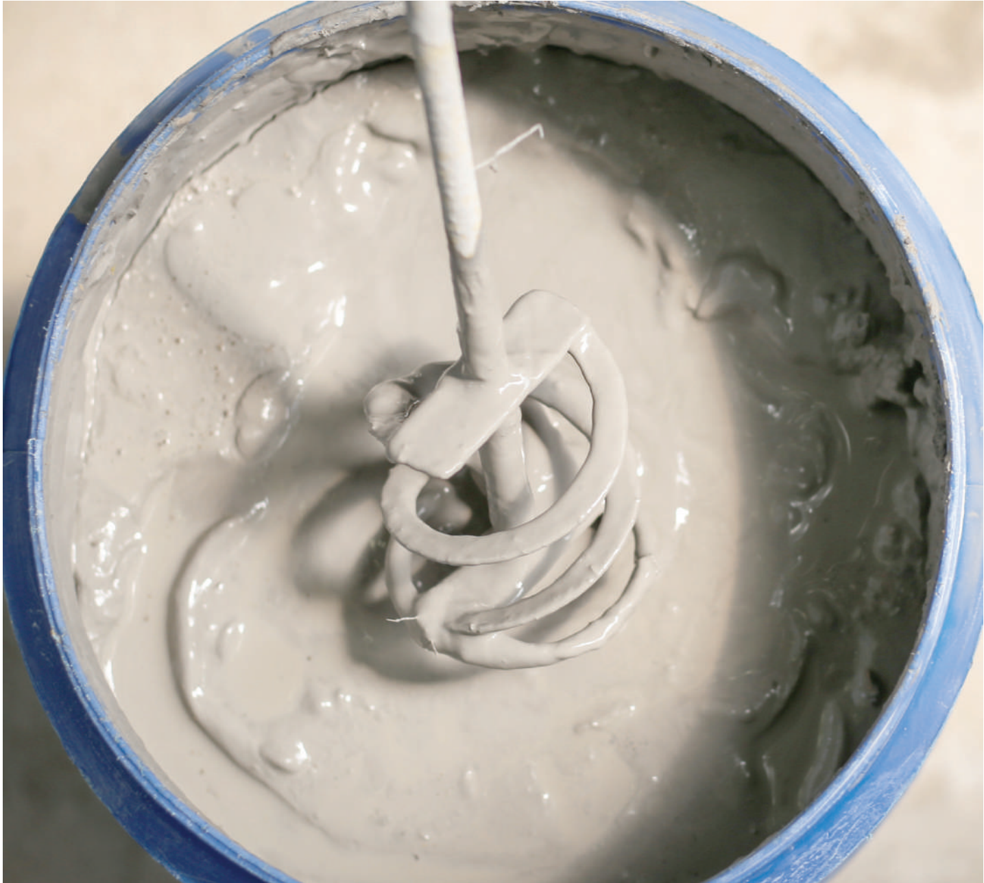
Unrefined clay along with combinations of refined clay and powdered or granulated non-plastic minerals are mixed to a creamy consistency with an electric mixer.
